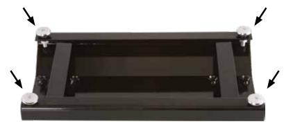
2. Attach the two support arms using the four M10x15 bolts. These may be tightened with a 5mm Allen wrench.
