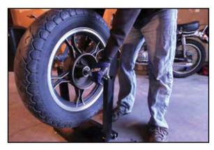
2. Slide the centering cones and rubber stoppers in place and tighten the set screws with a 2.5mm Allen wrench.
