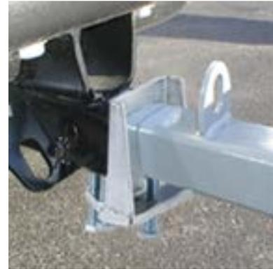
Step 5. The optional 8-1/2" small wheel adapter bolt (K) can be inserted into the front of the motorcycle rack to make the front wheel gap smaller.
