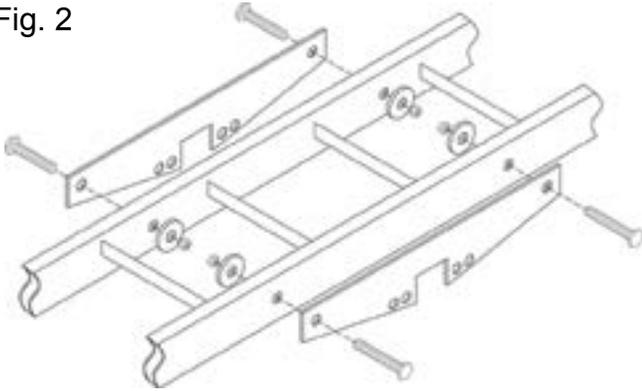
Step 4. The ramp (D) stores on either side of the motorcycle rack with the supplied wing nut, bolt, and nut assemblies (E).
